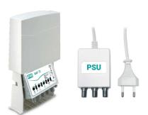
2-input (III+DAB, UHF) mast amplifier with 42dB gain and up to 116dB $\mu$ V output level on UHF band, separate VHF/UHF amplification with independent gain adjustment (0-15dB) for each input and low noise figure. T2 technology with UHF cut band for LTE 4G @790MHz and 5G @694MHz.
